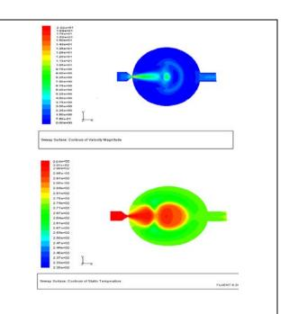
Fig. 3. velocity and Temperature distribution contour plots for 4 mm diameter nozzle with water input
