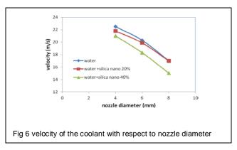
Figure 6 shows the velocity of the coolant with respect to nozzle diameter and different coolant used in the analysis. From the figure it is observed that the velocity of the water coolant is high when compared to the other coolant as the nano percentage increase there is a slight decreases in velocity. The maximum velocity is observed for the 4mm diameter in all the cases.
