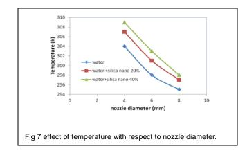
Fig7 shows the effect of temperature with respect to nozzle diameter and different coolant used in the analysis at the out let valve. It is observed that for the nano coolant of 40 % silica the heat observed is more than compared to other coolant. It is also observed that the maximum heat removed from the system when 4mm nozzle is used this may be due to high pressure the heat dissipation is more.
